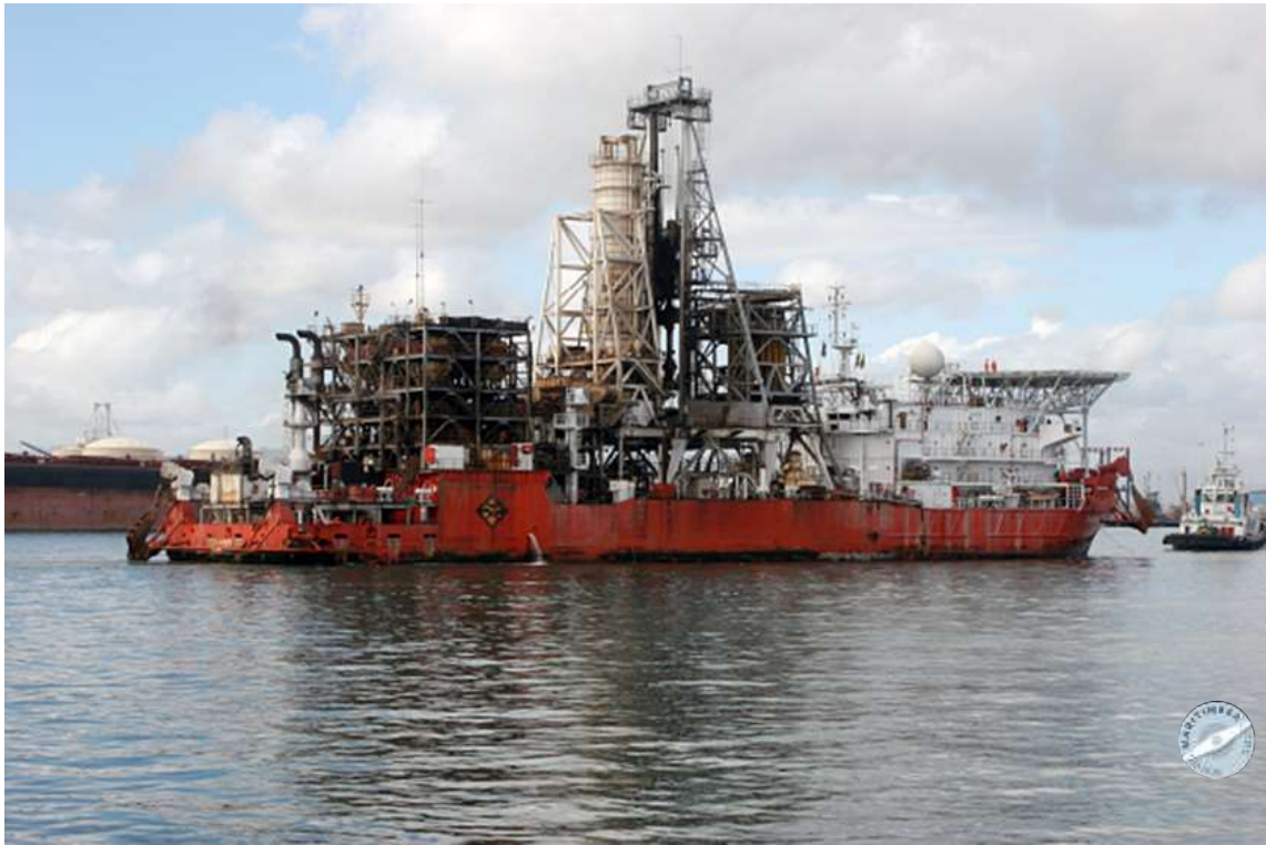
Figure 15: Gariep – Diamond recovery vessel using the vertical system
