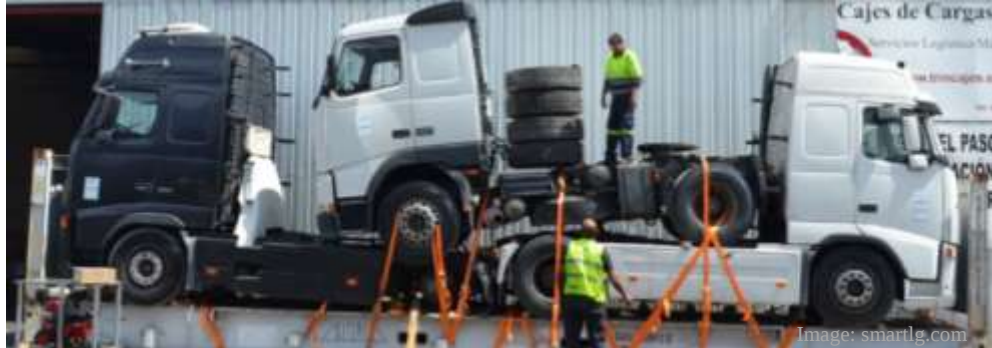
Figure 4: Three trucks loaded onto a 40ft flat rack collapsible container
