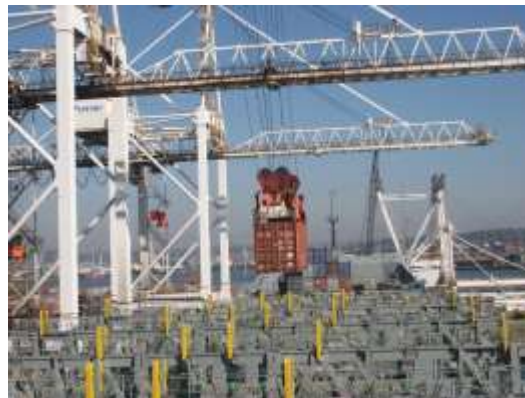
Figure 5: Containers being stowed in slots on a fully cellular container ship
