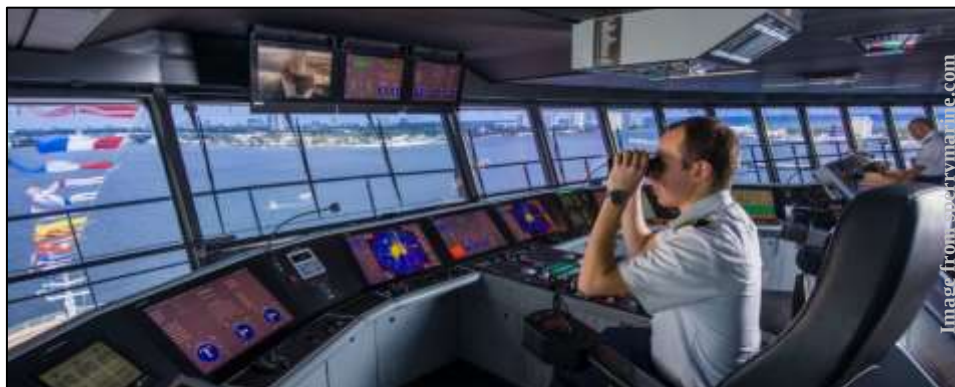
On the bridge of a ship. Notice the navigation system screens.
