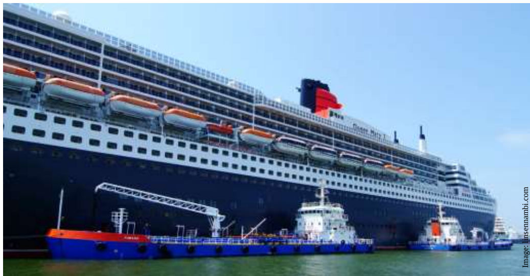
Figure 27: Fumana and Southern Venture berth alongside Queen Mary 2 to bunker the 345 meter long passenger ship.
