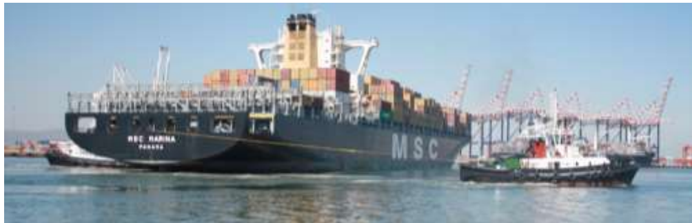
Figure 22: A containership being turned by a tug so that she can berth starboard side to (image from [1])
